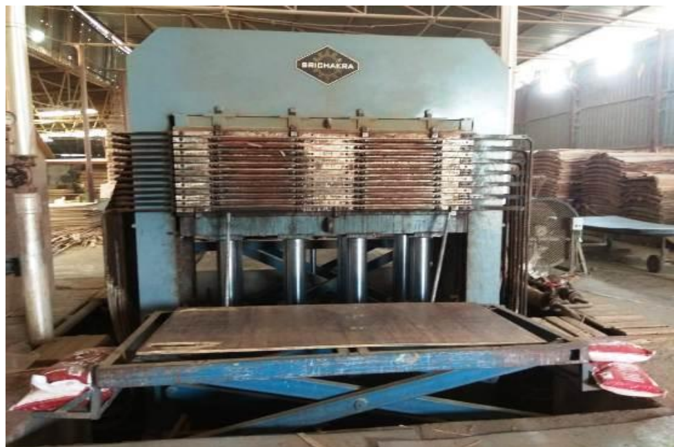
Pic 10: Compressing process of multiple panels in a daylight machine
