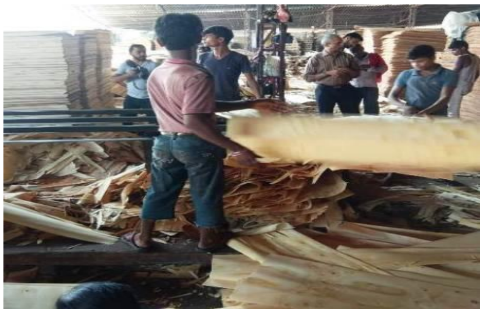
Pic 6: Defect removing & grading process on veneer
