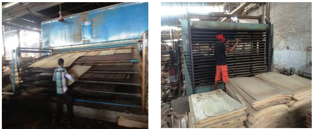
Pic 7: Veneer drying process
