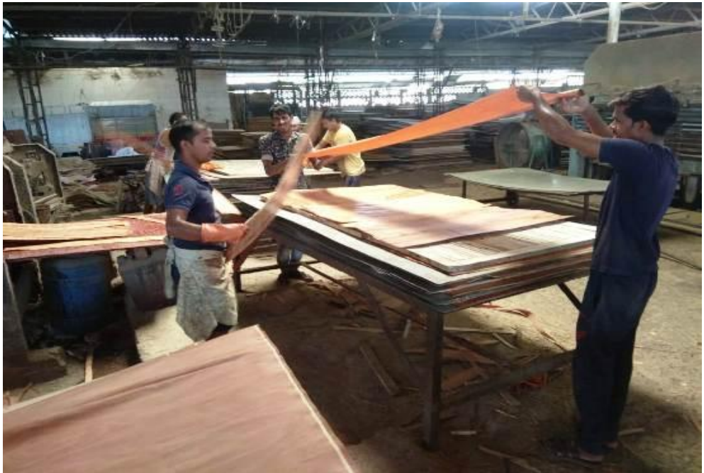
Pic 9: Veneer laying process for raw plywood
