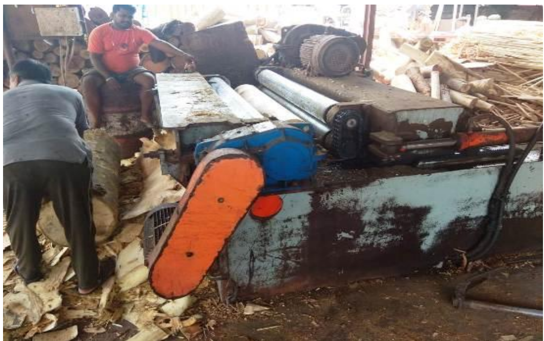
Pic 4: Debarking Operation on logs
