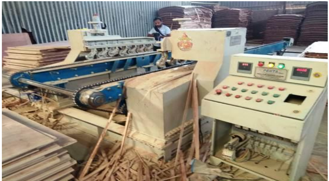
Pic 11: Plywood cutting & trimming process
