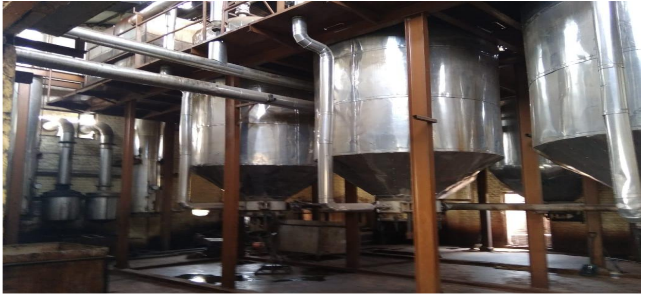
Pic 17: Autoclave for the extraction of hot liquid
