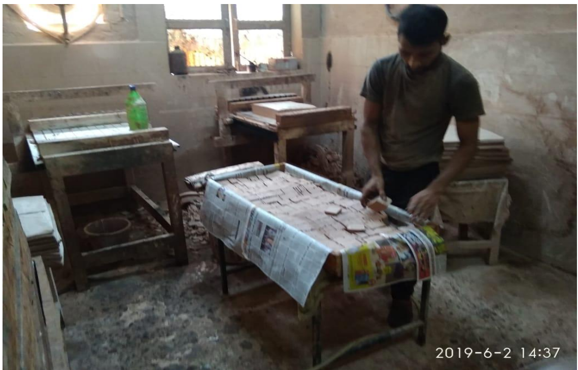
Pic 20: Catechu dried sheets cutting into Kattha biscuits
