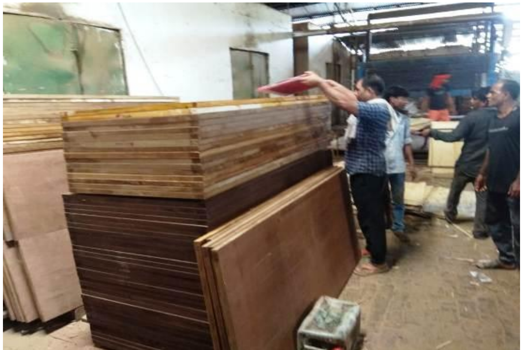
Pic 14: Branding of the plywood
