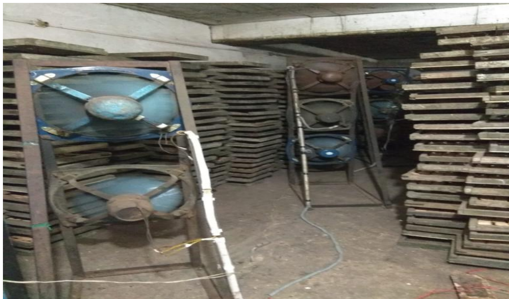
Pic 22: Ambient drying for hardening the Kattha
