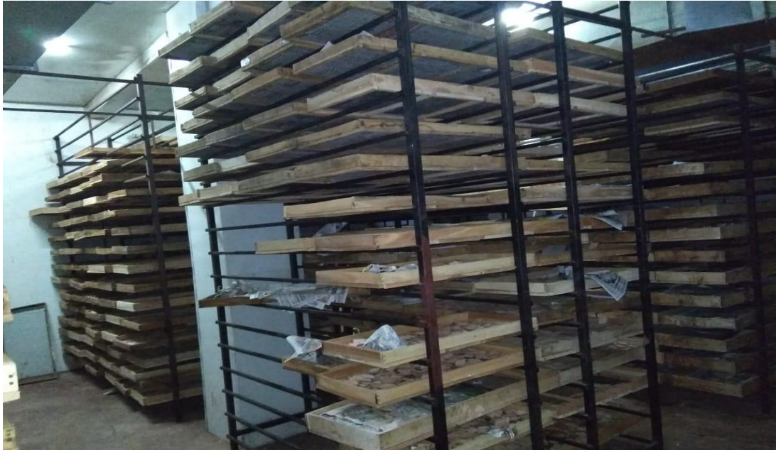
Pic 21: Cold drying chamber
