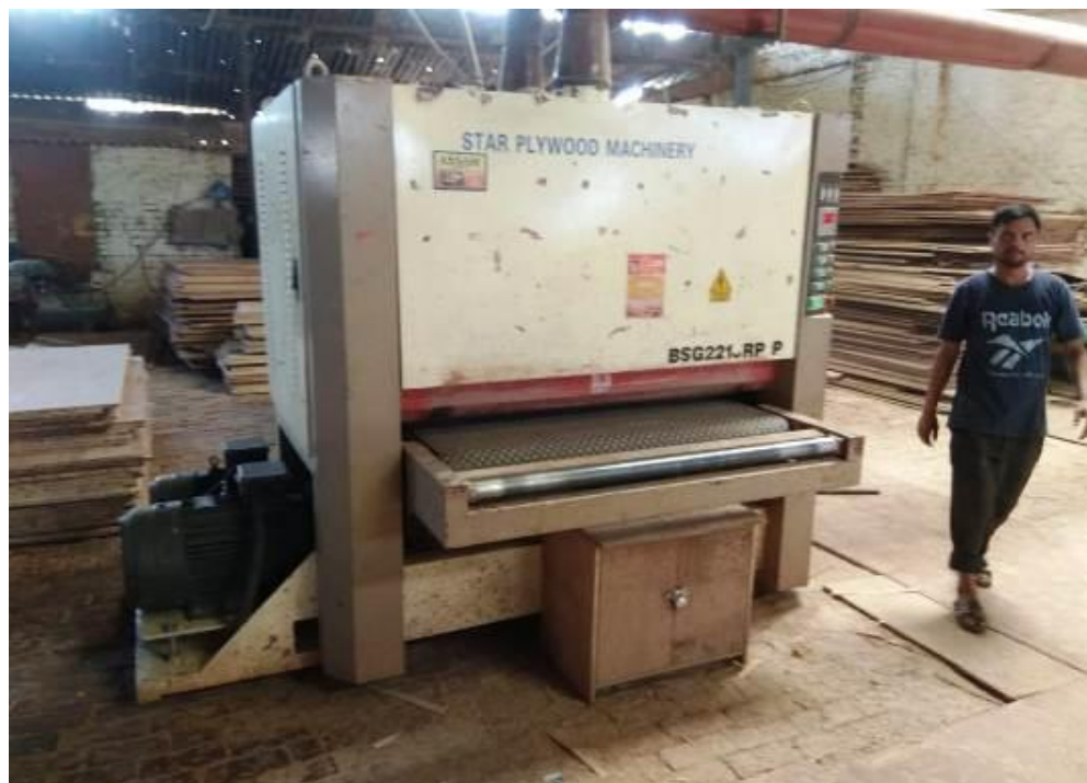
Pic 12: Sanding and Finishing process on plywood
